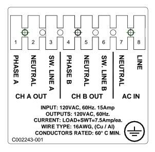
Figure 4-1: AC Connections
