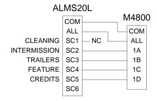
Figure 4-4: Slaving Signals to 2<sup>nd</sup> dimmer
