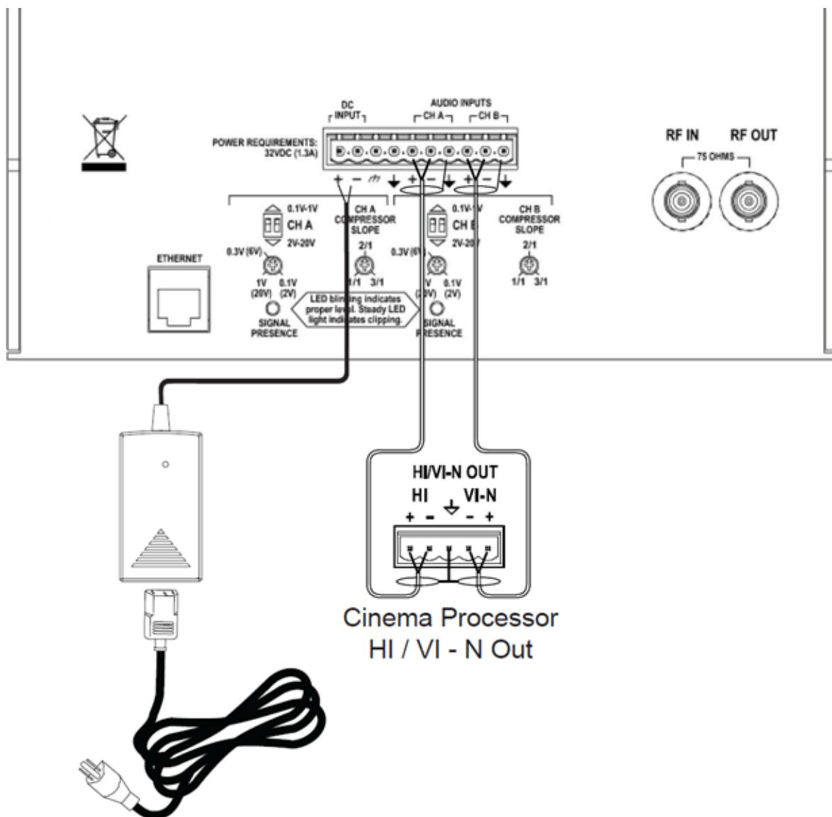
Figure 5-2: Power & Audio Connections
